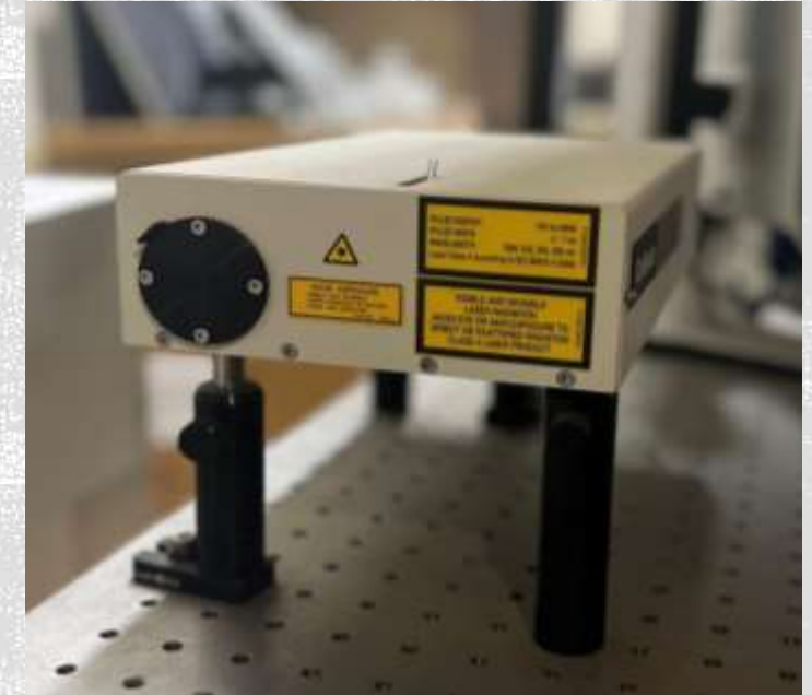
High Power Nd:YAG Laser, Minilite, ML11
