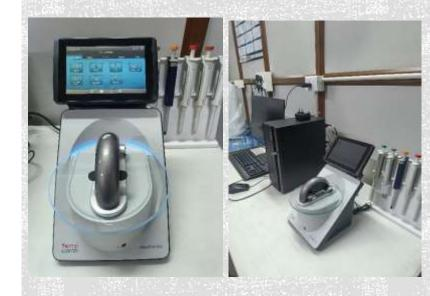
The Nanodrop Spectrophotometer is generally used to assess UV/visible light-based DNA, RNA, or protein quantities. These macromolecules in solution can have their absorbance spectra or individual wavelengths measured.
