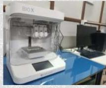
3D bioprinter uses biocompatible bioinks mixed with live animal cells to produce three dimensional structures mimicking invivo tissue arrangements.
